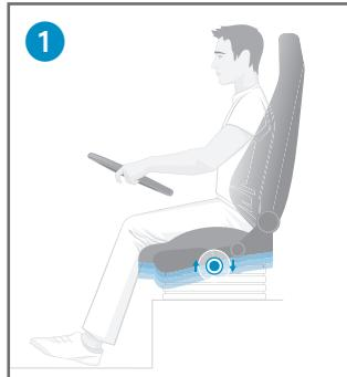
**Your RECARO Comfort-Plus:** For getting out of the vehicle, you should move the seat to the lowest position, using the switch (6) for express down. If you push the switch upwards again, the seat's memory function automatically moves the seat back to the previously set height position.
