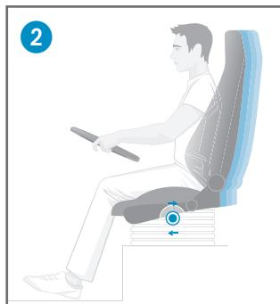
**Your RECARO Comfort-Plus:** With the new easy unlocking system (8, optional), a belt loop on the front edge of the seat cushion, it is easier for you to reach the length adjustment and are not forced to bend down to the vehicle floor.
